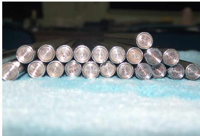
Figure 6: Cobalt-60 pencils from BRIT 52
